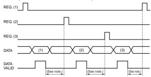
Note: Leave 20 ms min. between DATA VALID turning OFF and the REQUEST signal.
